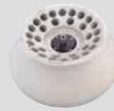
30x15 ml Angle rotor Max Speed 4500 rpm, Max RCF 2830 × g Radius 17 mm Item Number: 30314832 Auto rotor identification
