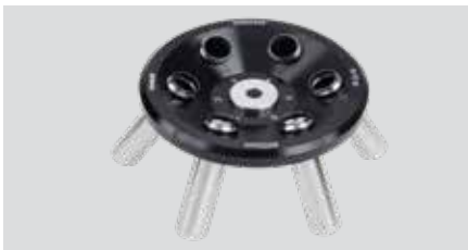
6 × 15 ml Angle rotor Max Speed 6000 rpm, Max RCF 3660 × g, Radius 17 mm Item Number: 30692838 Auto rotor identification
