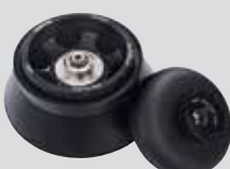
6x50 ml Angle rotor, Hi Max Speed 13000 rpm, Max RCF 15869 × g Radius 29 mm Item Number: 30314831 Auto rotor identification
