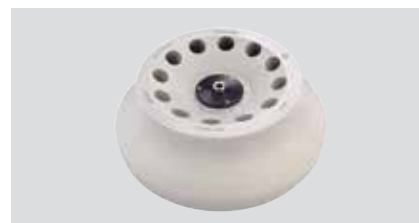
12x15 ml Angle rotor, ID Max Speed 6000 rpm, Max RCF 4427 × g Radius 17 mm Item Number: 30314834 Auto rotor identification ① The lowest temperature at max speed: -11.5°C
