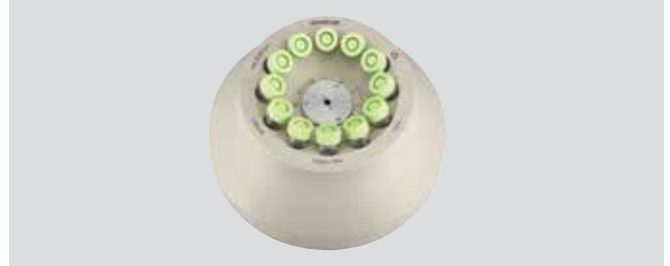
12 × 15 ml Angle Rotor Max Speed 6000 rpm, Max RCF 4427 × g, Radius 17 mm Item Number: 30130877
