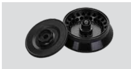
44x1.5/2.0 ml Angle rotor Max Speed 13500 rpm, Max RCF 17113 × g, Radius 11 mm Item Number: 30372718 Auto rotor identification ① The lowest temperature at max speed: 1 °C
