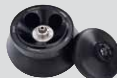
4x85 ml Angle rotor, Hi Max Speed 12000 rpm, Max RCF 14809 × g, Radius 38 mm Item Number: 30314827 Auto rotor identification
