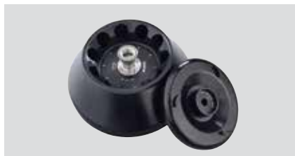
10x50 ml Angle rotor, ID Max Speed 7500 rpm, Max RCF 8174 × g Radius 29 mm Item Number: 30314829 Auto rotor identification ① The lowest temperature at max speed: 9°C
