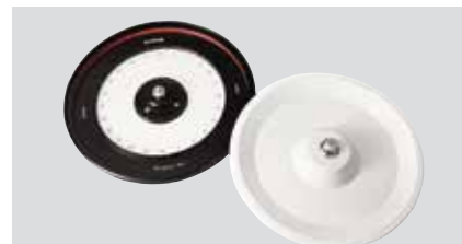
Hematocrit rotor, 24 × Capillaries Max Speed 12000 rpm, Max RCF 14811 × g Item Number: 30130881
