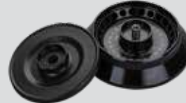
24x1.5 / 2.0 ml Angle rotor, Sealable Max Speed 15000 rpm, Max RCF 21379 × g Apply to FC5718 Max Speed 16000 rpm, Max RCF 24325 × g, Apply to FC5718R Radius 11 mm Item Number: 30642361 Auto rotor identification
