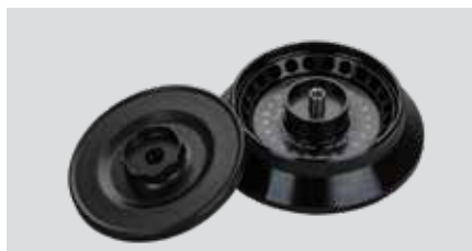
24x1.5 / 2.0 ml Angle rotor, Sealable Max Speed 14000 rpm, Max RCF 18624 × g Radius 11 mm Item Number: 30642361 Auto rotor identification
