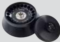
20x10 ml Angle rotor, Hi Max Speed 12000 rpm, Max RCF 15775 × g Radius 16 mm Item Number: 30314833 Auto rotor identification
