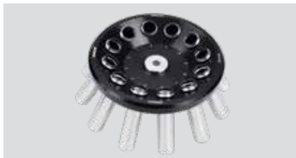
12 × 15 ml Angle rotor Max Speed 5000 rpm, Max RCF 3080 × g, Radius 17 mm Item Number: 30694907 Auto rotor identification
