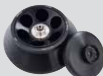
6x85 ml Angle rotor Max Speed 11000 rpm, Max RCF 15555 × g, Apply to FC5816 Max Speed 13000 rpm, Max RCF 21726 × g, Apply to FC5816R Radius 38 mm Item Number: 30314826 Auto rotor identification
