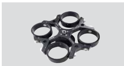
4x145 ml Swing out rotor Max Speed 4500 rpm, Max RCF 3350 × g, Radius 46 mm Item Number: 30314822 Auto rotor identification ① The lowest temperature at max speed: -7°C
