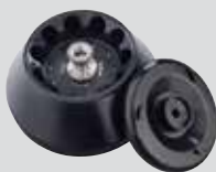
10x50 ml Angle rotor Max Speed 9000 rpm, Max RCF 11771 × g, Apply to FC5816 Max Speed 10500 rpm, Max RCF 16022 × g, Apply to FC5816R Radius 29 mm Item Number: 30314829 Auto rotor identification
