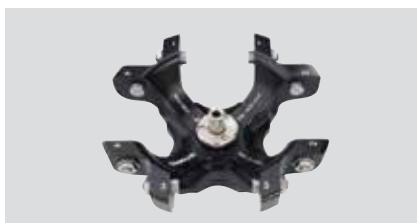
4x100 ml Swing out rotor, Sealable Max Speed 5000 rpm, Max RCF 3885 × g, Radius 40 mm Item Number: 30314823 Auto rotor identification ① The lowest temperature at max speed: -3°C
