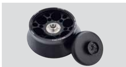
6x85 ml Angle rotor, Hi Max Speed 11000 rpm, Max RCF 13932 × g, Apply to FC5718 Max Speed 13500 rpm, Max RCF 20984 × g Apply to FC5718R Radius 38 mm Item Number: 30314825 Auto rotor identification ① The lowest temperature at max speed: 17°C
