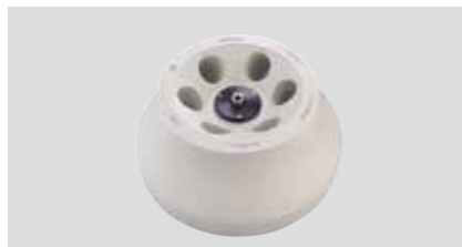
6x50 ml Angle rotor, ID Max Speed 6000 rpm, Max RCF 4427 × g Radius 29 mm Item Number: 30314830 Auto rotor identification ① The lowest temperature at max speed: -8°C
