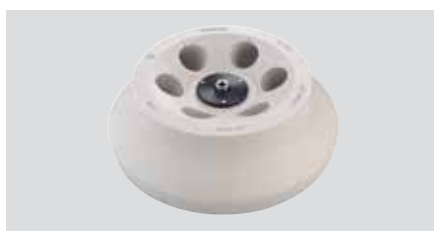
6x50 ml Angle rotor Max Speed 6000 rpm, Max RCF 4427 × g, Radius 29 mm Item Number: 30314830 Auto rotor identification
