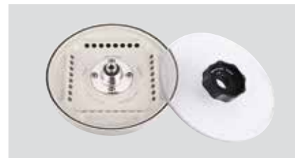
Angle rotor, 4x8-w PCR Strip Max Speed 15000 rpm, Max RCF 15342 × g, Radius 6.0 mm Item Number: 30130874
