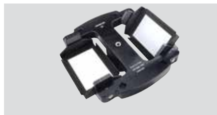
2x3 MTP Swing out rotor Max Speed 4500 rpm, Max RCF 2716 × g, Radius 11 mm Item Number: 30314824 Auto rotor identification
