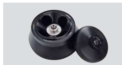
4x85 ml Angle rotor, Hi Max Speed 12000 rpm, Max RCF 14809 × g, Radius 38 mm Item Number: 30314827 Auto rotor identification ① The lowest temperature at max speed: 5°C
