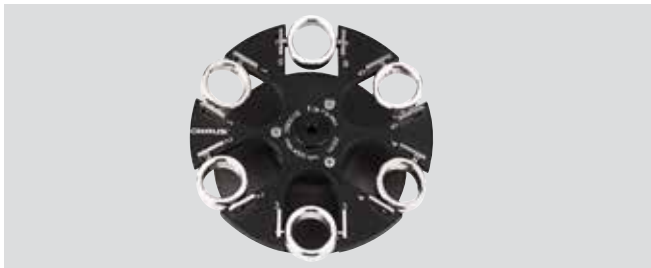
6 × 5 ml Swing Out Rotor Max Speed 4000 rpm, Max RCF 1878 × g, Radius 14 mm Item Number: 30130880
