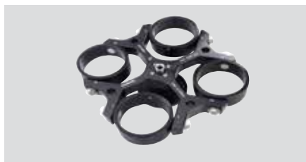
4x145 ml Swing out rotor Max Speed 4500 rpm, Max RCF 3350 × g, Radius 46 mm Item Number: 30314822 Auto rotor identification
