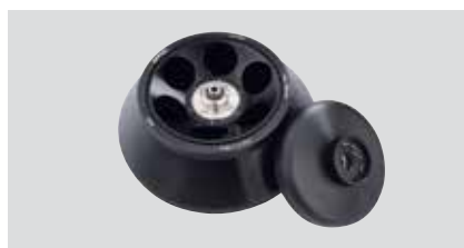
6x85 ml Angle rotor Max Speed 9000 rpm, Max RCF 10413 × g, Radius 38 mm Item Number: 30314826 Auto rotor identification ① The lowest temperature at max speed: -5°C
