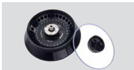
30x1.5 / 2.0 ml Angle rotor, Sealable Max Speed 12000 rpm, Max RCF 15131 × g Radius 11 mm Item Number: 30314836 Auto rotor identification
