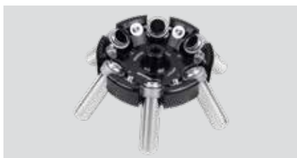
6 × 10 ml Angle rotor Max Speed 4000 rpm, Max RCF 2200 × g, Radius 16 mm Item Number: 30692865 Auto rotor identification
