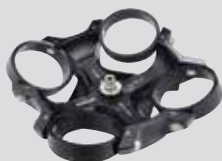
4x290 ml Swing out rotor Max Speed 4500 rpm, Max RCF 3780 × g, Radius 62 mm Item Number: 30314820 Auto rotor identification
