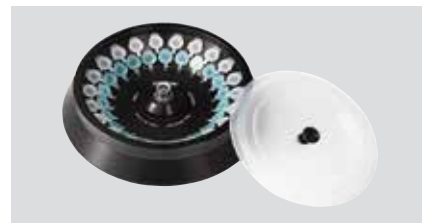
44 × 1.5 ml / 2.0 ml Angle Rotor Max Speed 13500 rpm, Max RCF 17113 / 17317 × g, Radius 11 mm Item Number: 30372717
