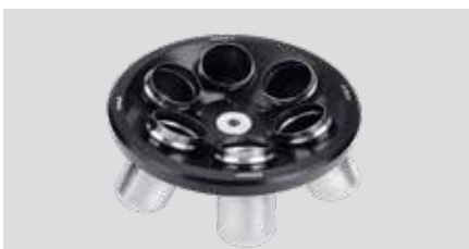
6 × 100 ml Angle rotor Max Speed 5000 rpm, Max RCF 3130 × g, Radius 41.5 mm Item Number: 30694814 Auto rotor identification
