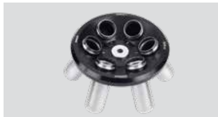
6 × 50 ml Angle rotor Max Speed 5000 rpm, Max RCF 2850 × g, Radius 28 mm Item Number: 30694811 Auto rotor identification
