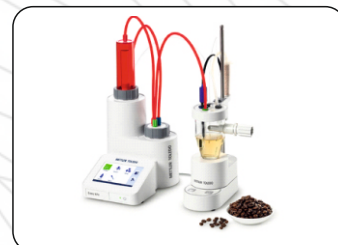
EasyPlus Titrator Easy KfV Water Determination Made Easy. Everything necessary for routine volumetric Karl Fischer titration from 100 ppm up to 100 % in food, chemical products, and other sample types
